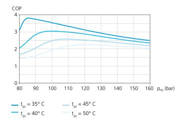
t<sub>ga</sub> = Gas cooler outlet temperature Limit conditions: isentrope compression
